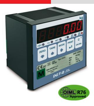
Multipurpose weight indicator/transmitter for panel mounting, 4 dependent or independent channels for direct reading and diagnostics of each connected load cell. The wide range of available interfaces, makes it easy to integrate the weighing with any automation system. CE-M approvable (OIML R-76 / EN 45501).
